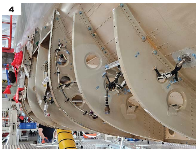
❶ Airbus built a new assembly hall for the rear center tank in Augsburg. ❷ The tank is an integral part of the fuselage structure. ❸ In Hamburg, the tank is integrated with Sections 15 and 17. ❹ Airbus extended the belly fairing to provide better crash protection.
