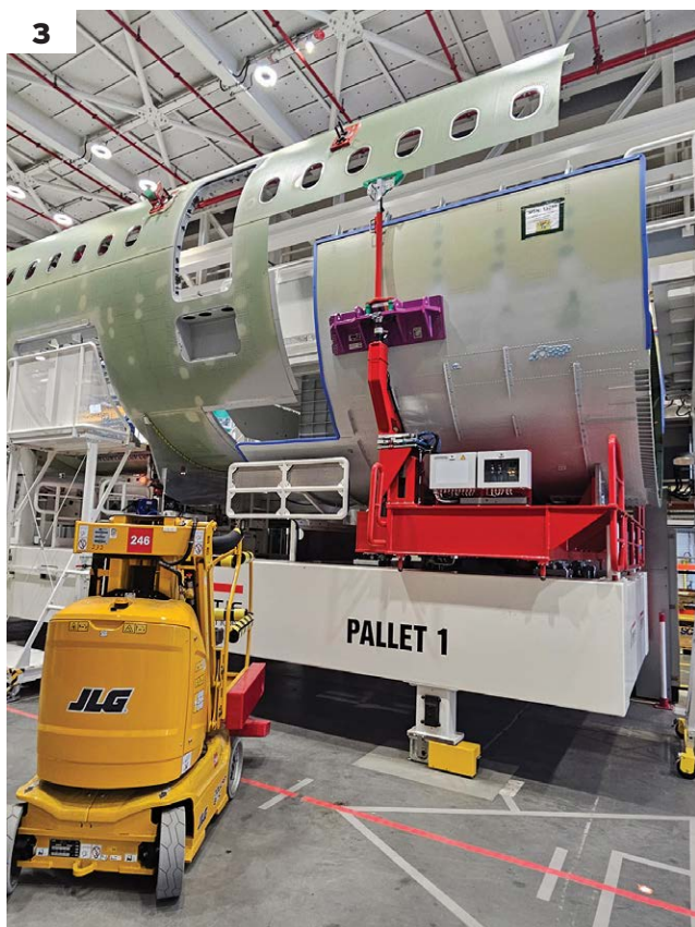
❶ Airbus built a new assembly hall for the rear center tank in Augsburg. ❷ The tank is an integral part of the fuselage structure. ❸ In Hamburg, the tank is integrated with Sections 15 and 17. ❹ Airbus extended the belly fairing to provide better crash protection.
