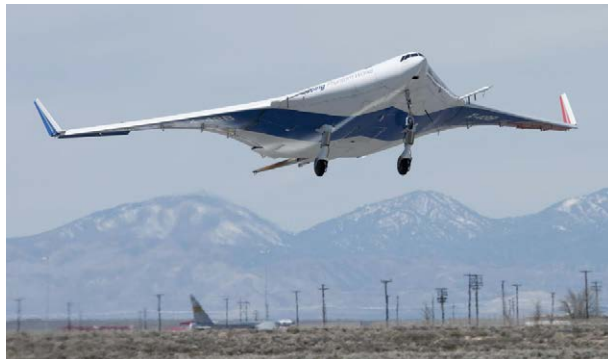
Liebeck's BWB vision took flight in 2007 as the 8.5%-scale NASA/Boeing X-48B demonstrator.
