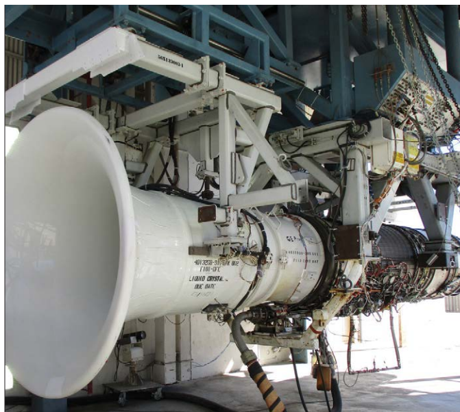
Dust ingestion durability tests of advanced high-pressure turbine blades for the compact RISE core are underway using an F110 engine.
