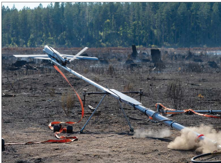
The U.S. Army experimented with the Aevex Aerospace Atlas (pictured) and other systems to assess the utility of launched effects munitions.
