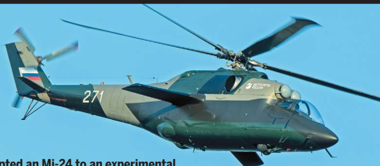
Mil adapted an Mi-24 to an experimental, high-speed system that reached 407 kph in 2016, a record for Russian rotorcraft.
