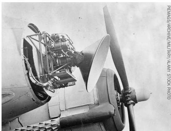
Microwave radar enabled the Royal Air Force Bristol Beaufighter Mk. VIF to intercept inbound German bombers at night.
