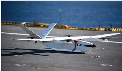
Delair's DT46 is a long-range fixed-wing uncrewed aircraft with optional vertical-takeoff-and-landing capability.
