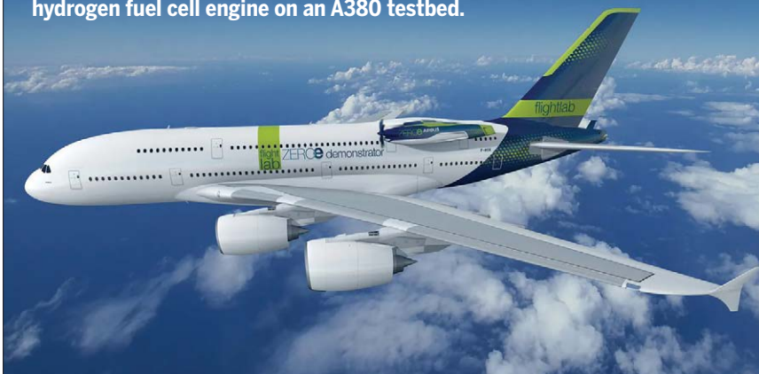
Airbus planned to flight-test a 2-megawatt hydrogen fuel cell engine on an A380 testbed.
