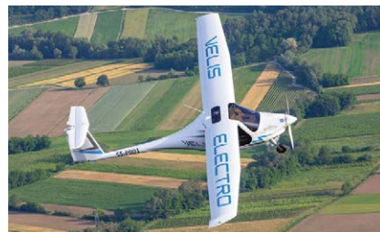
The Velis Electro is the first and so far only commercially available type-certified electric aircraft.
