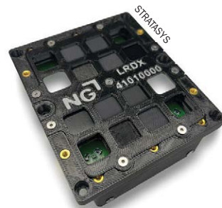
An FDM Antero 840CN03 radiation experiment housing contains radiation-shielding test samples.
