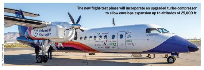
Pratt & Whitney PW123 turboprop on the Dash 8's right wing.
