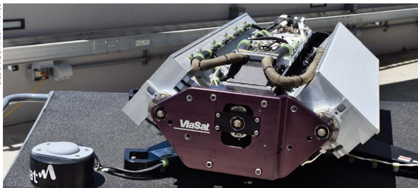
Viasat supplies dual, hybrid K_u -/ K_a -band satellite communications terminals, like the one pictured, on the Boeing 747 that serves as Air Force One.
