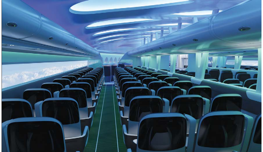
The wide single-deck main and aft cabin has three aisles, skylight windows and digital outside view display screens. The forward cabin has side windows.
