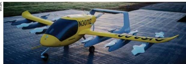
all-electric vertical-takeoff-and-landing (eVTOL) autonomous air taxi in the U.S. and New Zealand. Passenger-carrying trials are planned.
