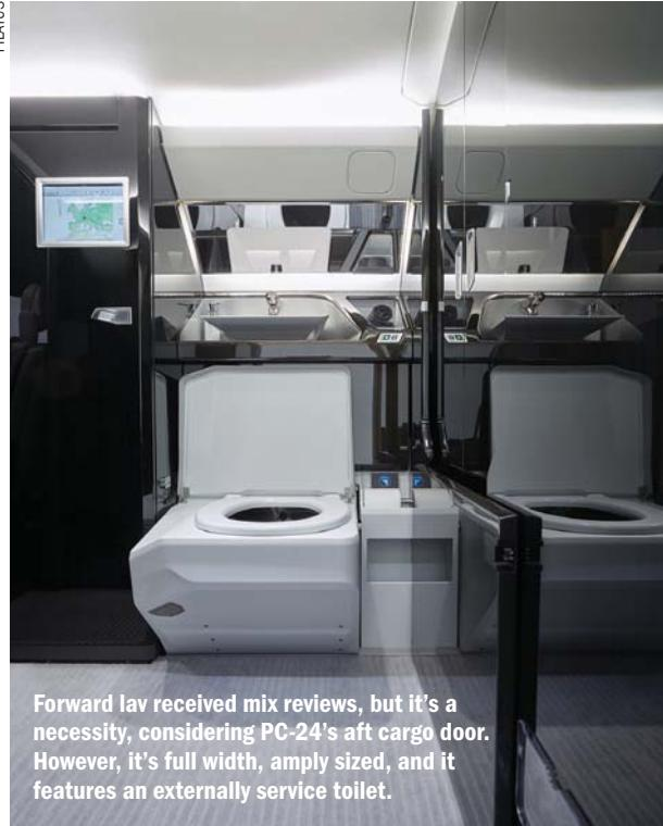
Forward lav received mix reviews, but it's a necessity, considering PC-24's aft cargo door. However, it's full width, amply sized, and it features an externally service toilet.
