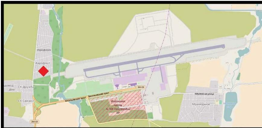
The peculiarity of Manas International Airport is that the ILS systems on both RWY approach courses have the same frequency (111.7 MHz) while their letter-codes are different. According to the available information, the system is configured in such a way that when the ILS for one approach heading is engaged, the ILS for the other approach heading disengages automatically.
