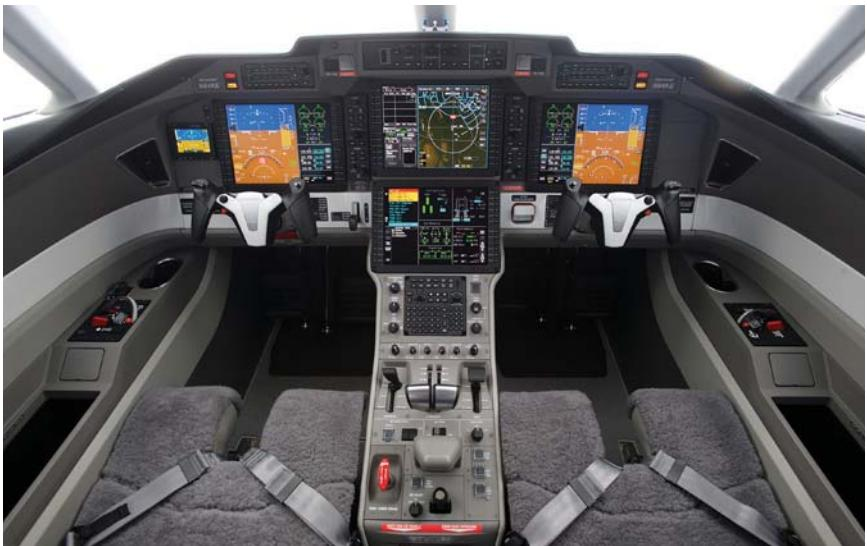
**Advanced Cockpit Environment [ACE], powered by Honeywell Apex, is quite similar to the flight deck of PC-12NG. Standard are autothrottles, LASEREF VI IRS, multi-sensor FMS and easy access to quick donning oxygen masks.**
