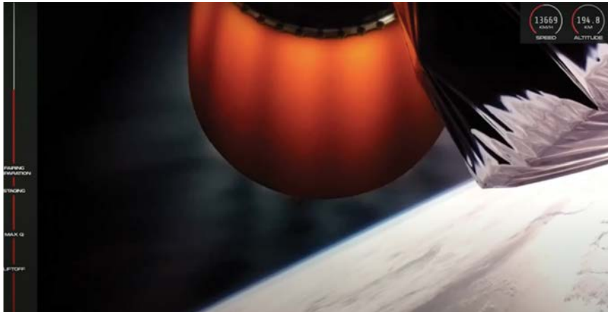
The glowing nozzle of the Electron rocket's second stage just before the video link was lost following the launch on July 4.
