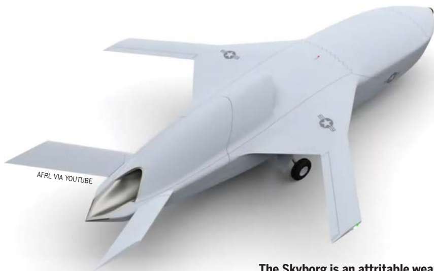
The Skyborg is an attritable weapon, which means key components such as the jet engine will be designed with a short service life.
