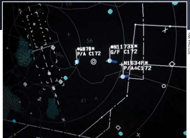
A tower controller monitored a display with ADS-B aircraft targets at Asheville Regional Airport in North Carolina.
