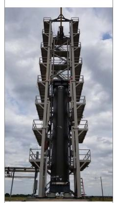
The first-stage LOX tank, the largest composite structure of its kind, passed acceptance tests in mid-May.
