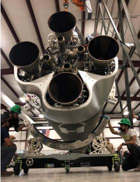
Four Reaver Stage 1 engines will boost Firefly's Alpha launch vehicle with a combined thrust of more than 165.000 lb.
