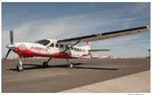
MagniX and AeroTEC flew a Cessna 208B Caravan converted to all-electric propulsion for the first time on May 28 from Moses Lake, Washington (page 48).
