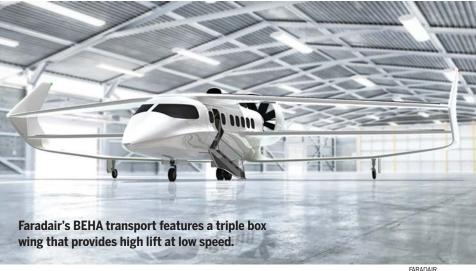
super-STOL (SSTOL) hybrid-electric aircraft for regional mobility using DEP and powered lift. He is working with a team from the Massachusetts Institute of Technology (MIT) that has been studying SSTOL as an alternative to eVTOL for urban air mobility (UAM).
