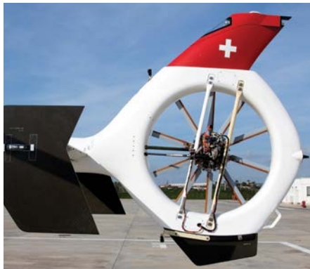
The Maestro shrouded tail rotor helps improve safety on the ground, particularly during loading and unloading with the engine running.
