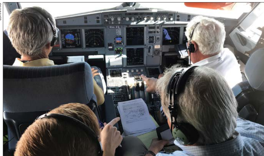
Pilots and engineers with American Airlines and L3Harris conducted certification flight tests of the SafeRoute+ ADS-B In system on the carrier's Airbus A321 at Phoenix Sky Harbor International Airport.
