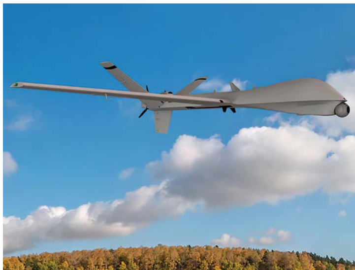
An image released by the Israeli military depicts a concept for a laser interceptor pod for rockets mounted on the nose of a generic UAV design.
