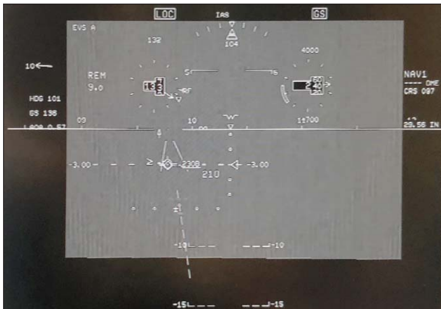
The best technology is useless if you don't know where to look. In this photo, the 1,000-ft. roll bars (horizontal approach lights) can be seen below the synthetically drawn runway, but only if you are looking for them.
