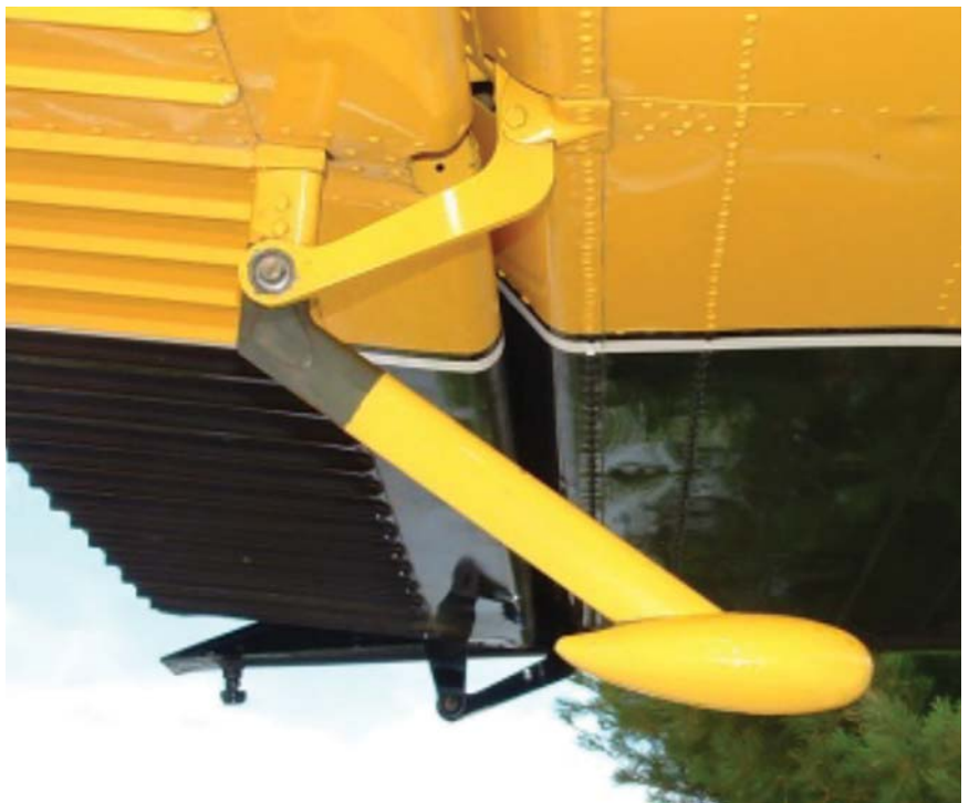
Additional mass in the form of weights is often used to prevent wing/aileron flutter as well as to improve the balance of the flight control force. These should be checked for proper installation and security during preflight inspection.
