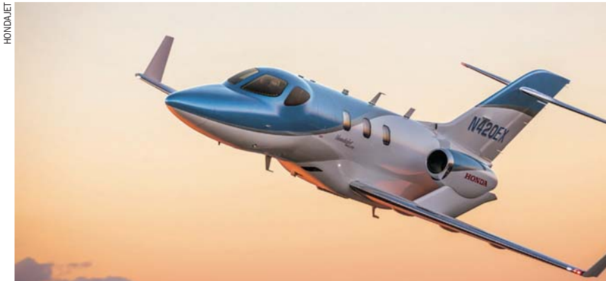
Adding 104 lb. more usable fuel and an aggressive drag reduction program boosts range by more than 200 nm. We recorded 390 KTAS while burning 570 lb./hr., beating book predictions.
