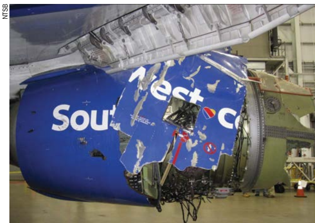
Separation of the fan blade at its root on Southwest Airlines Flight 1380 sent blade fragments into the engine fan case and compromised the outer fan cowl structure.
