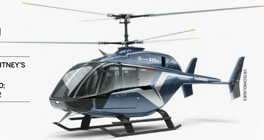
Russian Helicopters believes the VRT500 will find a niche in the urban air mobility mission, thanks to its coaxial configuration.
