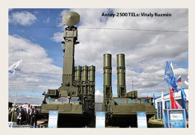
First shown at the MAKS Airshow in 1992 and cleared for export in 1993, the S-300PMU-1 / SA-20A Gargoyle (originally, SA-10D) introduced a vastly improved, fully mobile search radar, updated engagement radar and TELs and a new missile with far greater range. It could engage aerodynamic targets at altitudes down to 10 meters and intercept ballistic missiles with ranges up to 1,000 km, traveling at speeds up to 2,800 m/s at distances up to 40 km from the battery.
