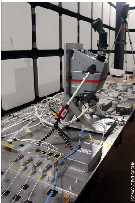
An inceptor system for the Typhoon is ready for electromagnetic compatibility testing in one of the Faraday Center's anechoic chambers.
